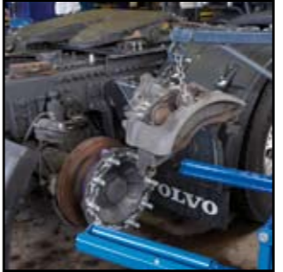
Dismounting of calipers - to spare the mechanic the heavy lifting jobs
