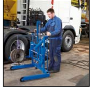
Dismounting of disc brake - easy and ergonomically correct lifting
